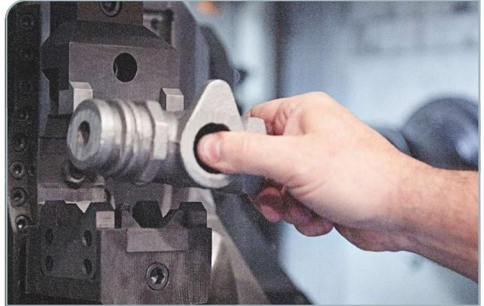
∴ Workpiece blanks enter the machine workzone through a load/unload station. It can accommodate manned or automated operation.
