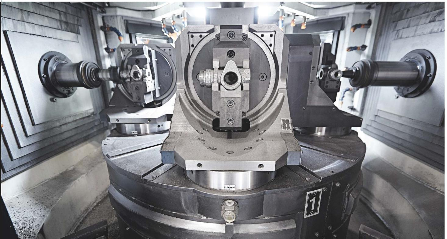
In 2005, Porta introduced its solution to the dedicated machine versus a flexible machine in the form of the Multicenter. The thinking was to bridge the dedicated machining technology designed around a specific part with a machining center platform that could easily be retooled as part mixes changed.
